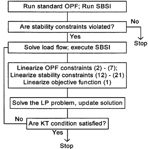
Fig. 1. Overall procedure for stability constrained OPF.
