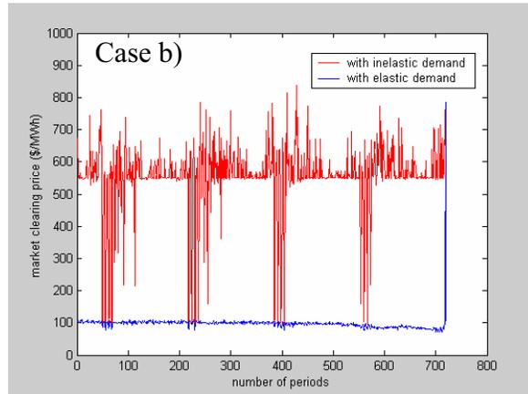
**Figure 4. Two typical simulation results with inelastic demand without demand-side participation (red line) and with elastic demand with demand-side participation (blue line). Case a) shows the results in a more competitive market than that for Case b).**
