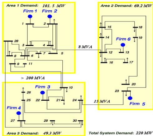
**Figure 3. Modified IEEE 30 bus system with six suppliers. Capacities of lines connecting Area 1–Area 2 and Area 3–Area 2 are lower than those of other lines.**
