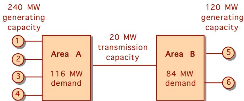
**Figure 1:** Transmission Network Block Diagram
